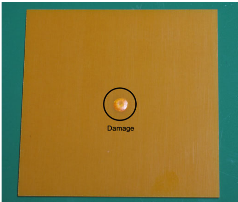
Photo 3(c) In a mere 10 seconds, the phenolic resin laminated sheet was deformed.
